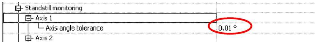
**Fig. 54 Standstill monitoring - Axis angle tolerance**
